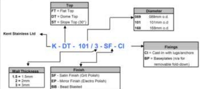
K-DT-101/3-SF-2 = Kent Stainless Dome Top Bollard, 900mm above ground, 300mm below ground, 101mm outside diameter with 3.05mm wall, Satin Polish Finish, Cast in with Lugs.
