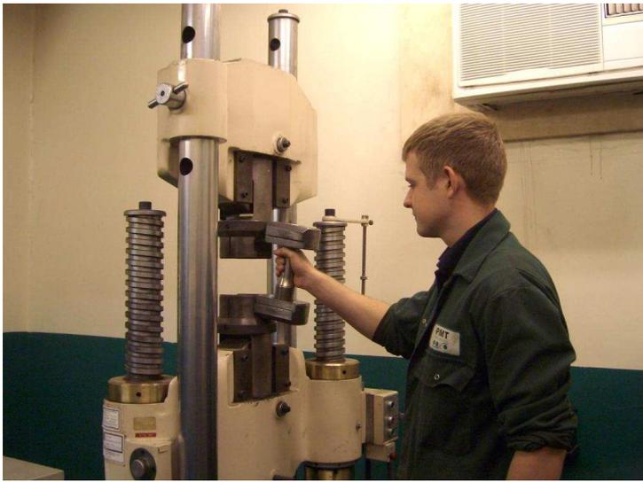
**Test Bar Tensile Testing Equipment**
