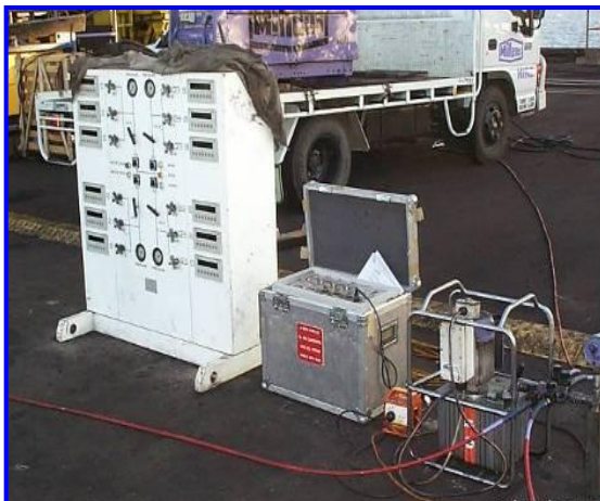
Hydraulic Power Pack and Weighing Equipment Readout
