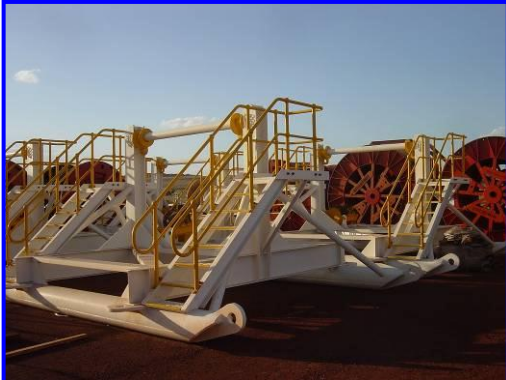
Hoist Rope Skids
