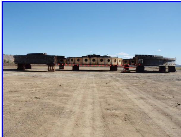
Marion 8200 Dragline Tub Relocation Wesfarmers Curragh to BMA Blackwater
