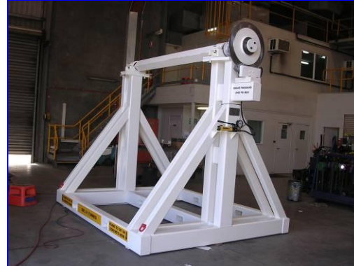
Conveyor Belt Support Stand
