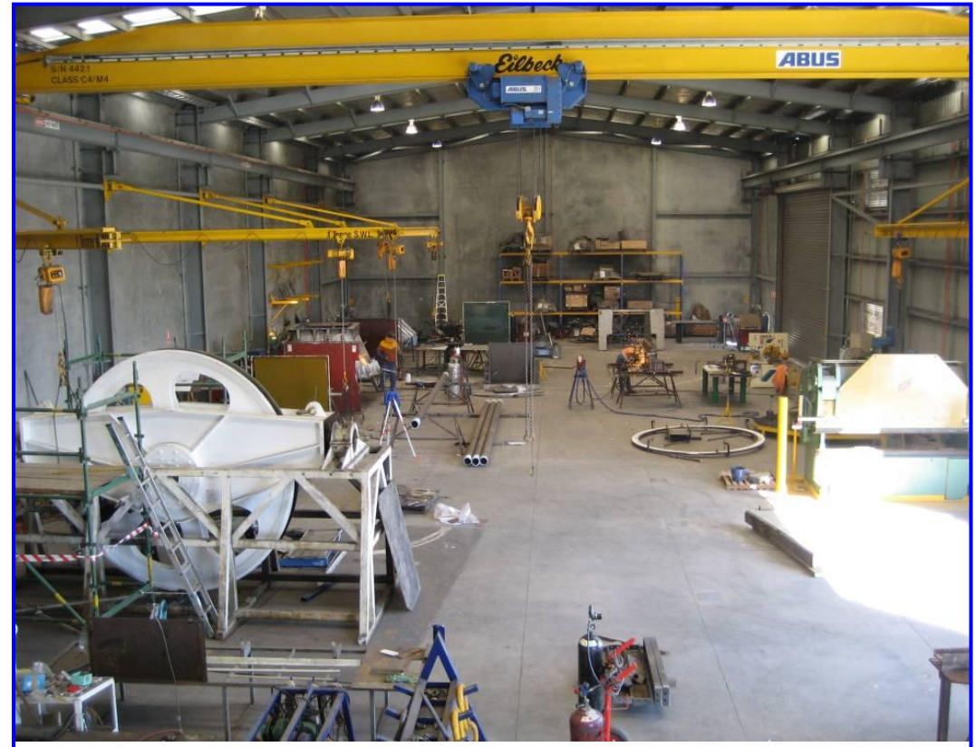
Workshop complete with 25T overhead crane & 10 off 600A welding outlets
