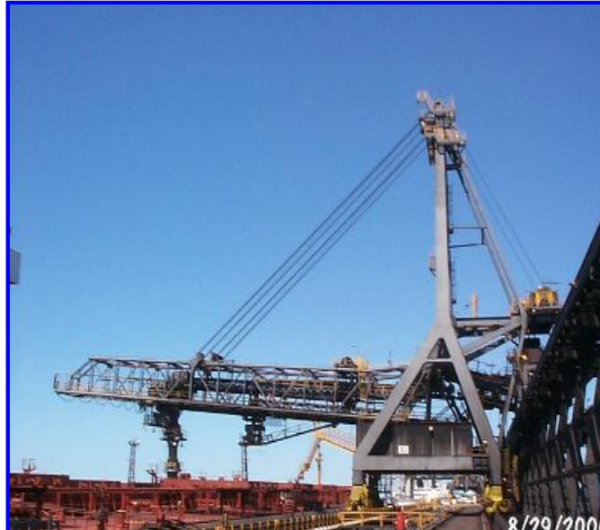
Weighing and Center of Gravity Testing Execution of in situ weighing of 1200T rail mounted ship loader four bogies simultaneously at Dalrymple Bay
