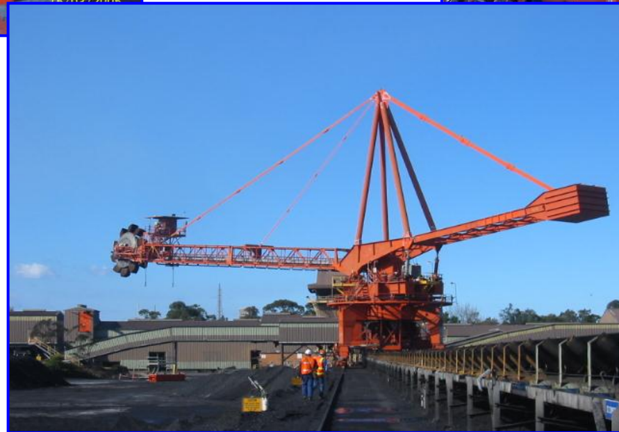
Port Waratah Coal Services Reclaimer 1 Return to Service Upgrade Bucketwheel, Shaft and Drive Unit Replacement, Slew Bearing Changeout, Rocker Arm Repairs and Luff Cylinder Changeout
