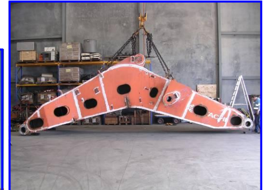
Excavator Boom Refurbishment
