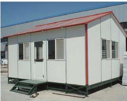
1. 9910 type house is a modular house which width is fixed at 5048mm and length can be extended by adding number of 1224mm based on 2200mm.
