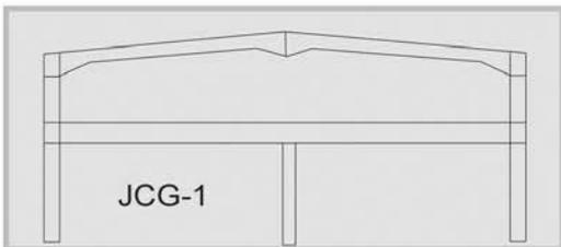
Light steel structure system with interlayer, column of constant cross-section, roof beams with column bases of rigid connection of styles of DMG-1, maximum span of floor beams  $L \leq 12M$ .
