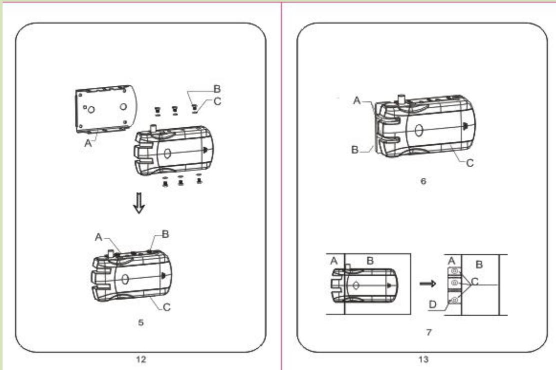
Assemble the remote control lock and fixation board into one with 4 M5×6 hexagon bolts (Diagram 5).
