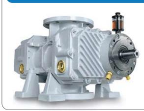
The Roots-Type Pumps belong to the group of positive displacement pumps. Two symmetrical pistons having an eight ligure, housed in the pump body, rotate in opposite directions with no contact neither between each other nor with the pump body, meshing continuously. The pistons are driven by a set of gears with synchronised rotation, which guarantees friction free movement. Capacity available from 200 m<sup>3</sup>/hr to 15000 m<sup>3</sup>/hr
